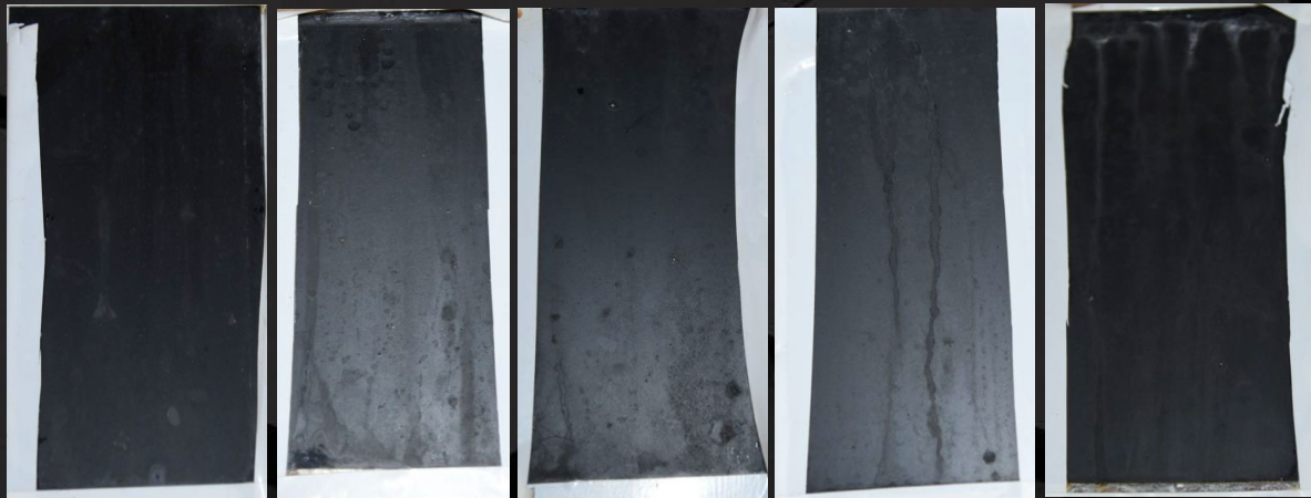
Images of THERMAL-XR® coated plates after 30,000 hours of salt spray testing
